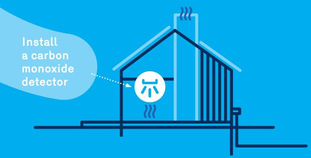
Carbon monoxide is an odourless and invisible gas that may be produced by a fuel-burning appliance, like a natural gas appliance, if combustion is partial or incomplete. This may happen if the maintenance of your appliance is neglected. If not detected, carbon monoxide can cause serious health problems, even, in rare cases, death.
